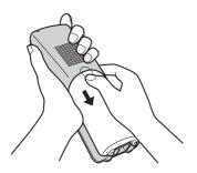
2 Insert the battery (1), and press it down until it snaps into position (2). Then close the handset cover (3, 4).
